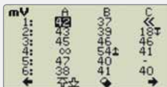
Grid Batch feature facilitates fast surveying for Half-Cell readings
